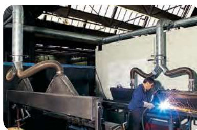
Slotted extraction hoods in the automotive industry
