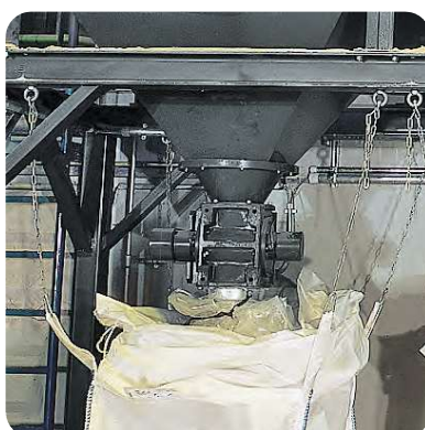
Removal through rotary valve
