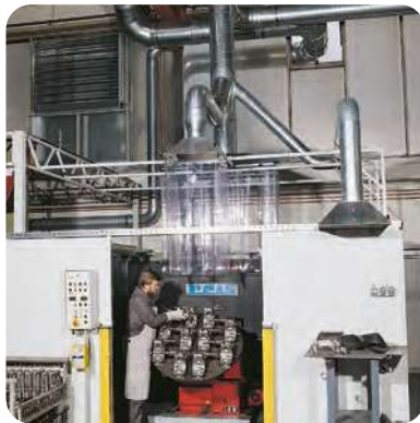
Extraction at a robotic welding station
