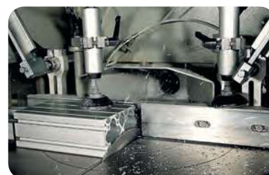
Extraction of aluminium shavings
