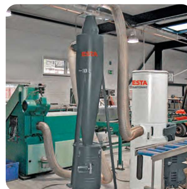
Cyclone pre-separator ZA-160 application photo
