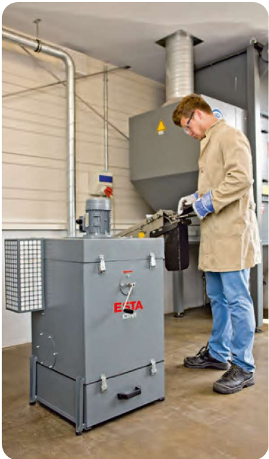
OM-8 connected to a belt sanding machine
